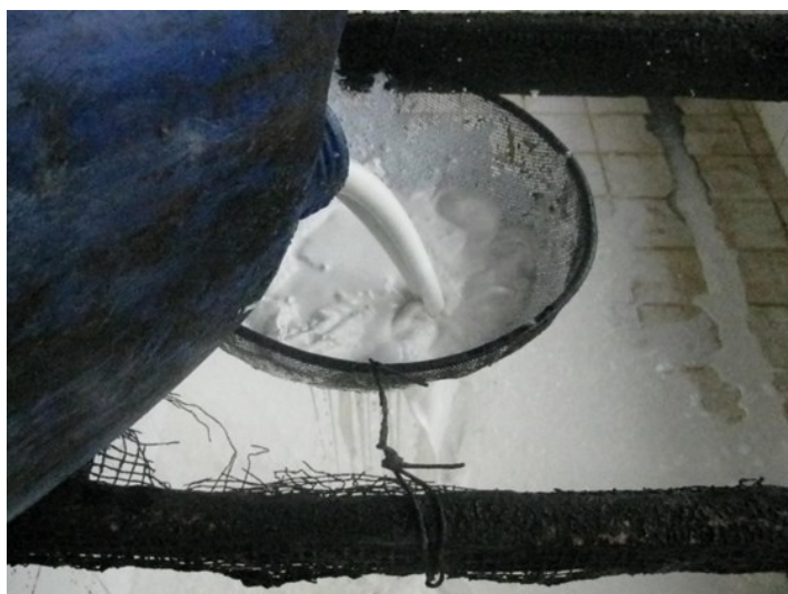
Figure 5. Newly collected latex being transferred to the tiled vat
