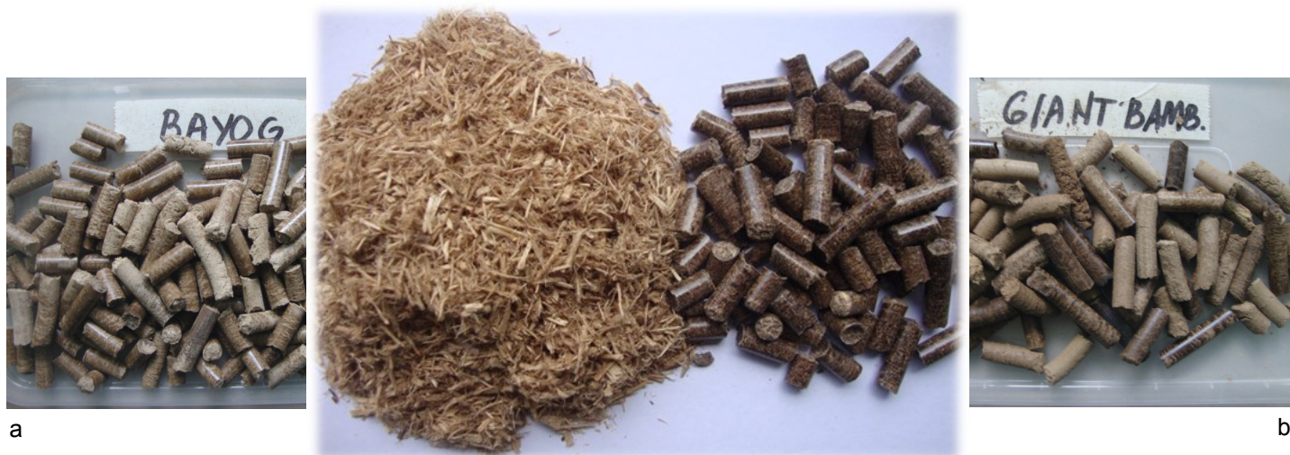
Photo of wood pellets sample made from (a) Bayog and (b) Giant Bamboo.
