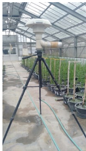
Fig. 2. Micrometeorological Instrument for Near Canopy Environment of Rice (MINCER) placed inside the glasshouse used in the three trials. This is the instrument used to monitor the environmental conditions inside the glasshouse.
