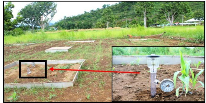
Figure 3. Tensiometer installed inside lysimeter tank.
