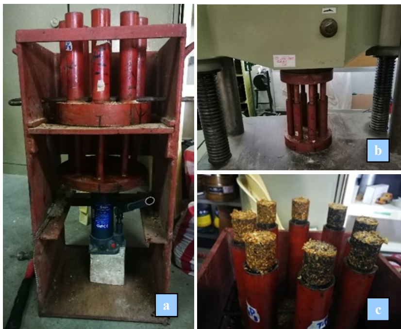
Figure 1. a) The mold placed under the piston attached to the UTM; b) The mold above the extruder pushed by a hydraulic jack; and c) Briquettes extruded through the machine.
