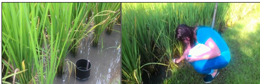
Figure 2. Measurement of evaporation using the stilling well and a floater with pointer.
