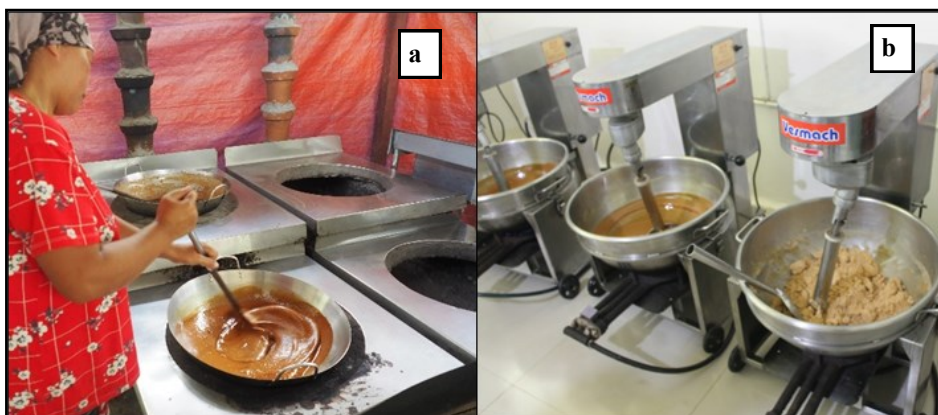
Figure 2. Manual (right) vs. mechanical (left) crystallization process.
