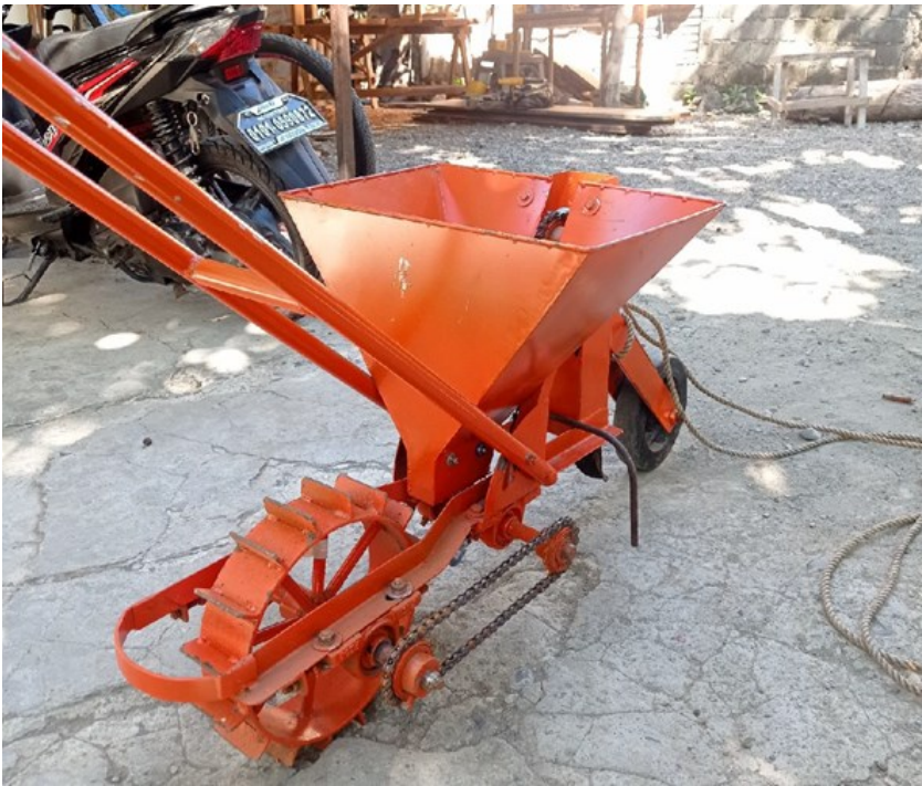
Figure 2. The fabricated garlic planter.
