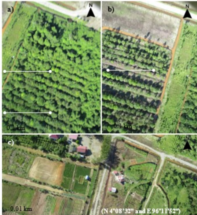
Figure 11. A digital photogrammetric UTU captured from VTOL-UAV camera: (a) blur image, overlapped speed; (b) open exposure image; and (c) Bright captured image at 150 m.
